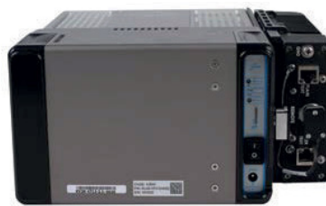
Voyager 2 rear showing UBI-2590 battery, DC input and HAIPE power
